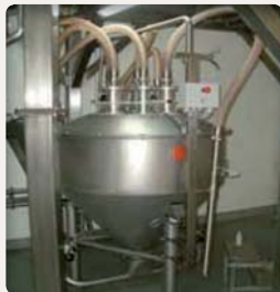
Vacuum pneumatic conveying with integrated «weight gain» scale. This pattern is specially designed for the suction of multi-components
